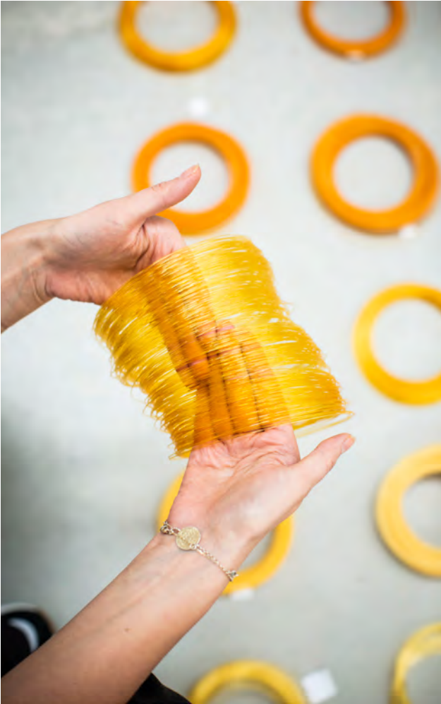
Filament for textile production coloured with Dunaliella Salina, 2019
